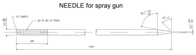
NEEDLE should be machined from 1/8-inch diameter BRASS ROD (SAE 41)
